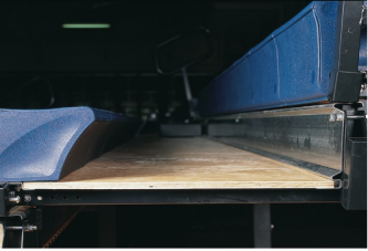
E. Full-Length Captured Decking Decking is captive in the riser beam and rests on the nose, firmly secured by the seat bracket. This system provides a stiff, secure walking surface with no exposed hardware. MAXAM is the only telescopic gym seat that utilizes transverse decking, using decking materials in accordance with their industry span rating. Load tested and independently verified, MAXAM's support system provides an enhanced level of performance, safety and stability.
