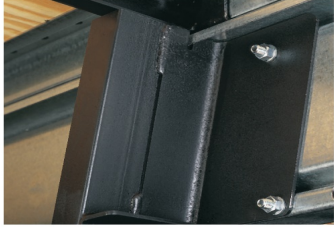
F. Slant Frame Design Load-tested and certified for 30 tier single stack sections up to 25' 6" (7772 mm), our slant frame design delivers improved cantilever strength and capacity. It also simplifies the installation process, reducing downtime for the facility. Critical support areas are all fastened with bolts, lock washers and hex nuts. Only MAXAM incorporates a steel to steel connection where the frame meets the wall, creating a stronger union and a safer gym seat.
